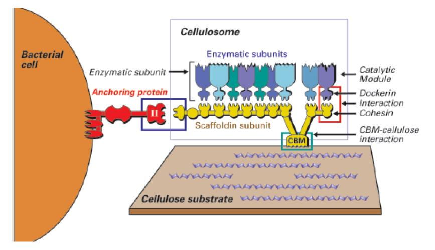
**Cellulosomes** can be designed with complementary enzymes to form a single multi-enzyme complex. Cellulose hydrolysis rates were shown to be 2.7- to 4.7-fold higher compared with purified enzyme preparations.
