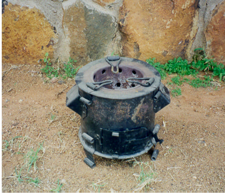
Figure 4.7: Charcoal stoves used at Mpala Ranch. (a) Metal Jiko . (b) Kenya Ceramic Jiko (KCJ) (c) Loketto . In each stove, charcoal burns in the upper container and the lower chamber is used for lighting the stove and collecting the ash.
