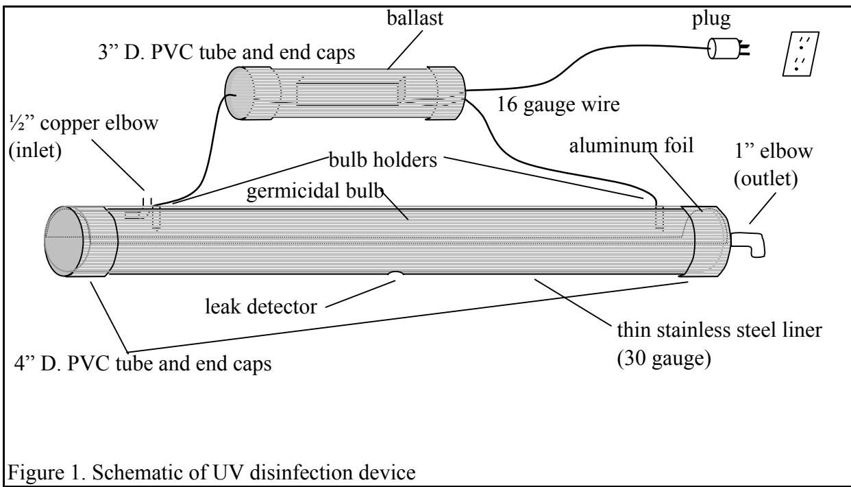
Figure 1. Schematic of UV disinfection device
