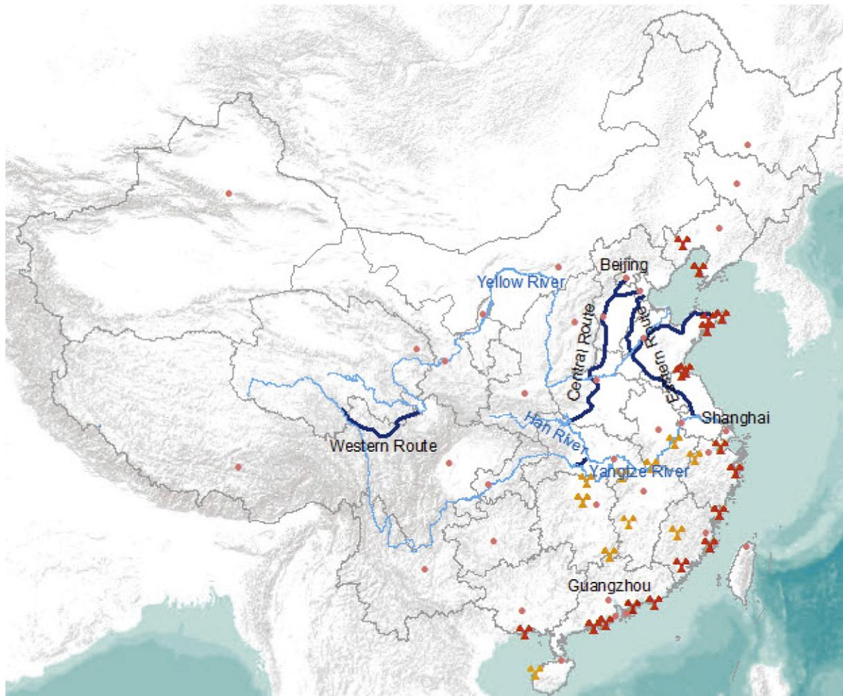
**Fig. 1.** Chinese nuclear fleet by 2030 [3–5] and Eastern, Central and Western routes of the South-to-North Water Transfer Project [6]. The three routes are drawn in dark blue. Red crosses represent nuclear plants hosting reactors appropriate to nuclear desalination in 2030, while yellow crosses indicate not appropriate nuclear plants.
