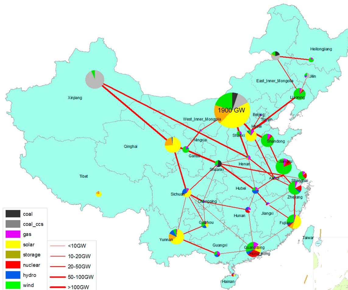
**Figure 4.** Infrastructure, generation, and transmission capacity needed to achieve an 80% carbon reduction in 2050. All represented lines are new transmission expansion. Inner Mongolia emerges as a major center of clean-energy generation thanks to the combination of its location (a few hundred kilometers from major demand centers) and high-quality renewable energies.
