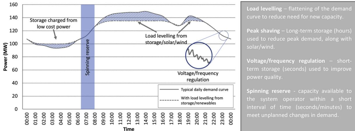
Fig. 2. Grid services that can be provided by electric vehicles and renewables, based on a 24-h demand curve for Barbados (Hohmeyer, 2015).
