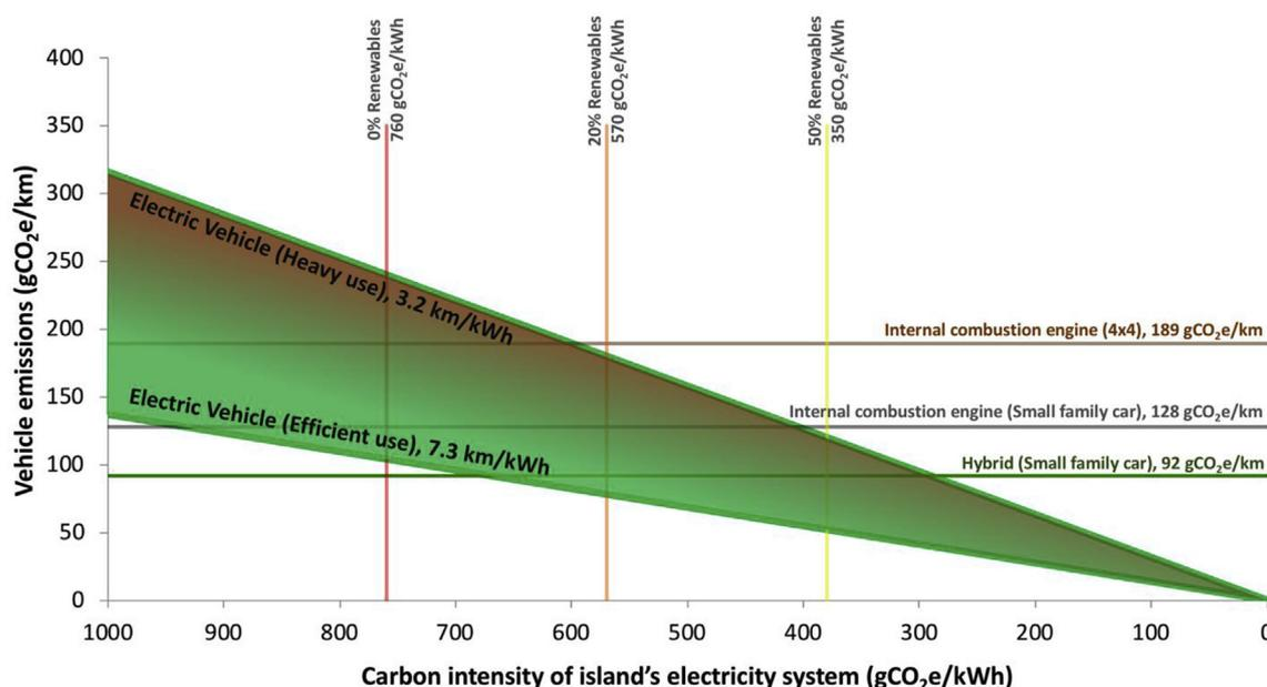
Fig. 3. Emissions of different vehicle types and impact of carbon intensity of electricity supply for an island energy system.
